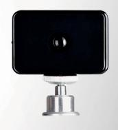
For measurement of luminance [cd/m²] and color coordinates (x,y,Y) conforming to CIE standards.
