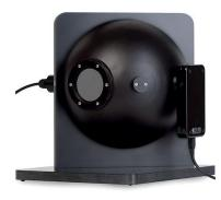
The GL OPTI SHERE 205 is designed for the measurement of radiant power and luminous flux of LEDs and other light sources compilant with the recommendation of the CIE Technical Committee published in Technical Report CIE 127:2007. The sphere is suitable for IESNA LM-79-08 compilant measurements.
