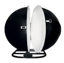
The GL OPTI SPHERE 2000 has been designed for the measurement of luminous flux and radiant power of LED Luminaries and big LED modules as well as for other light sources compliant with the recommendation of the CIE Technical Committee published in Technical Report CIE 127:2007. The sphere is suitable for IESNA LM-79-08 compliant measurements.
