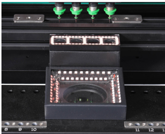
4 placement cameras + 1 high precision
